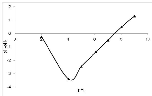
Figure 1.  $pH_{zpc}$  of GUL. (Powder addition method)
