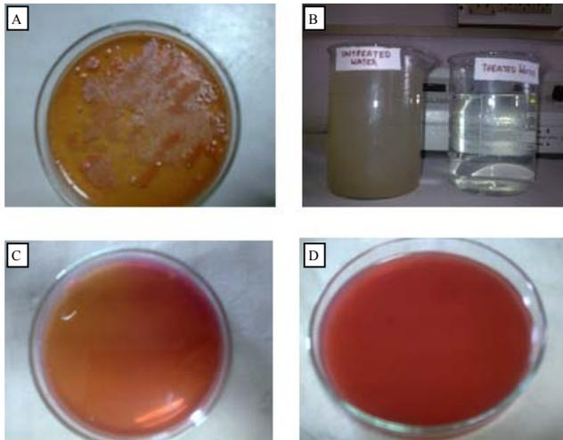
**Figure 4.** Coliforms inactivation by water clarified with *Dolichos lablab* and solar disinfection. A) Coliform count in turbid water, B) Treatment with natural coagulant (NC), C) Coliform count after NC treatment, and D) Coliform count after solar disinfection.
