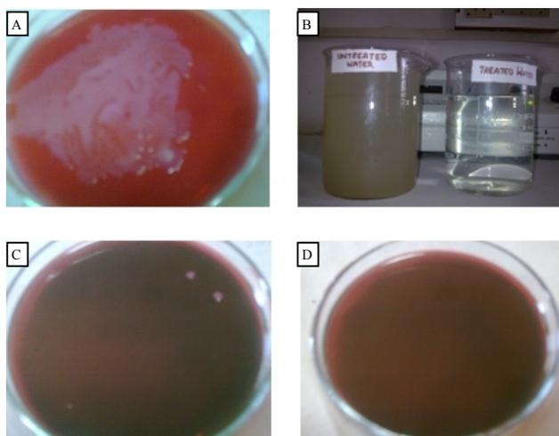
**Figure 3.** *E. coli* inactivation by water clarified with *Dolichos lablab* and solar disinfection. A) *E. coli* count in turbid water, B) Treatment with natural coagulant (NC), C) *E. coli* count after NC treatment, and D) *E. coli* count after solar disinfection.
