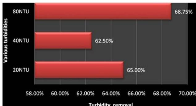
**Figure 2.** Percentage of turbidity removal at various turbidities with *Dolichos lablab* at dosage of 200 mg/500 ml at settling time of 60 min.
